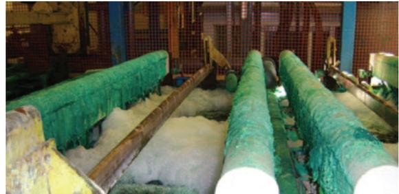
AIR AGITATION [NOTE CONTAMINATION OF TANK AND ADJACENT SURFACES.]
