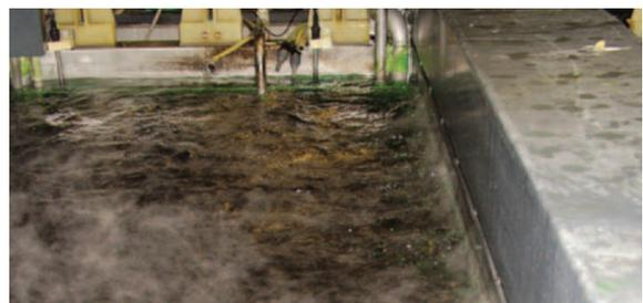
AGITATION BY PUMPED FLOW EDUCTORS [NOTE THE CLEAN ADJACENT SURFACES.]
